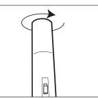
Remove the battery cover at the bottom of the microphone by twisting it counterclockwise.
